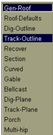
The operator is presented with a number of options for inserting the roof geometry. The first, **Dig-Outline**, allows the operator to “snap” to the extents of the building outline from a plan that has been imported into the system via DXF or DWG format. As many builders and designers these days are using CAD for their drawings, this option is very quick. Alternatively, this method can be used in conjunction with a digitizing tablet.
