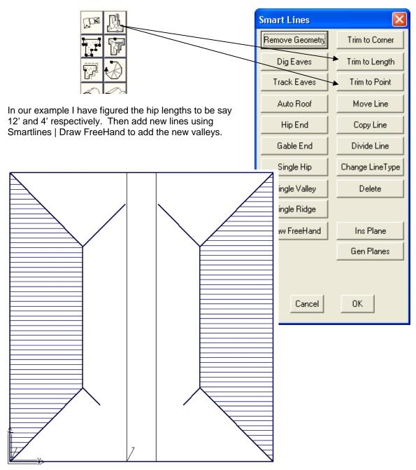
We also need to decide what type of line is used at the intersection of the cricket and the main roof -I used an Apron. Remember to use the middle mouse button to 'snap' to the intersection of the corner lines.
