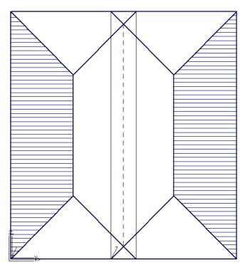
Now we must determine where to draw the extents of the cricket. This information is hardly ever easy to extract from an architect's plan (they often don't know either), so you will have to scale it off the plan. We need to trip the hip lines to suit the cricket and insert new lines that will be the valley at the edge of the cricket.
