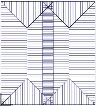
Now use **Mod-Roof > Advanced > Intersect planes** to cut out the crossing over pieces of each roof. This is not essential, but with some roof shapes of this type, it will do a lot of the tidy up for you.
