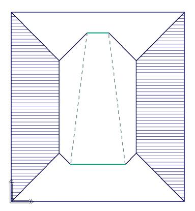
Now use **Smartlines > Insert Plane** to reinsert the roof planes that are required. To insert the planes at the top and bottom, you will have to delete one of the eave lines as they do not connect. Then use **Smartlines > Trim to Point** to make a closed loop of the roof plane area.
